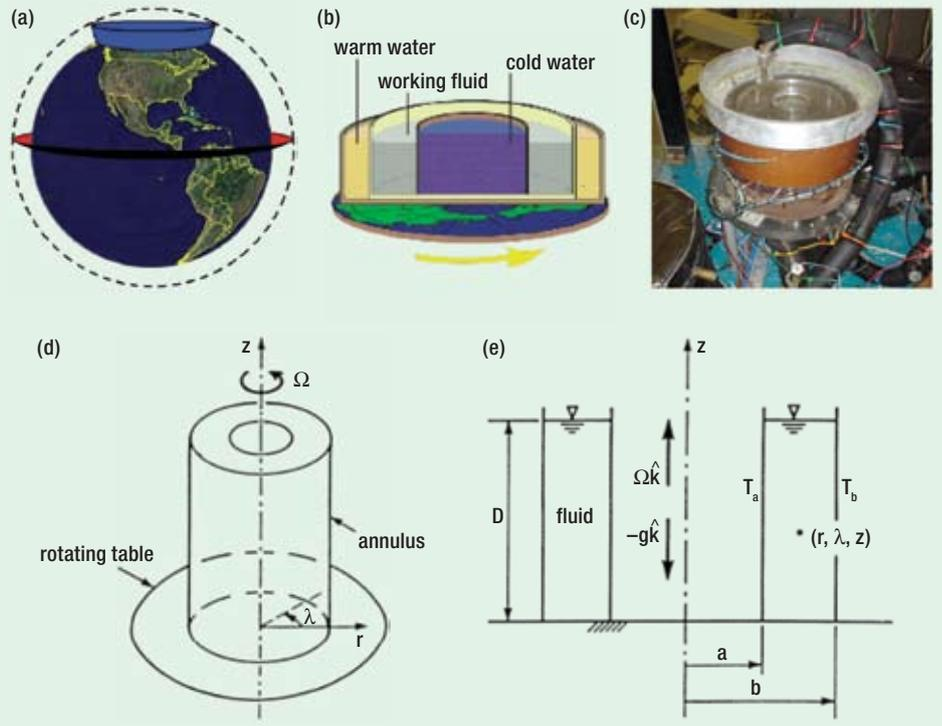
experiments at the University of Chicago used water in a dishpan, mounted on a rotating table. A heat source was provided near the rim, and in some experiments there was a cold source in the centre. The idea was that the rim simulated the equator and the centre was the North Pole.
